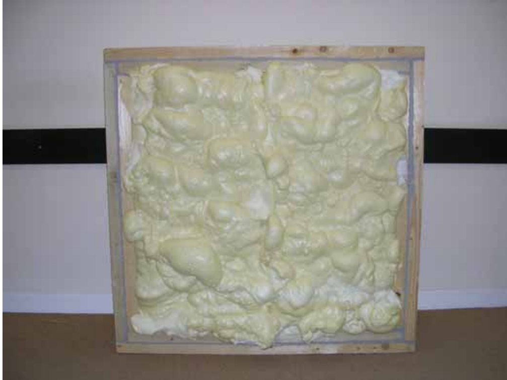
Photograph 2 – Test Sample 2 Foam with surface trimmed level
